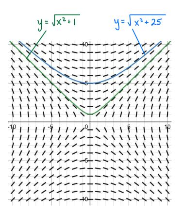
Two solutions to the DE  $y' = \frac{x}{y}$ . The sloped lines are tangent to the curves at each point (x,y).
