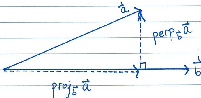
The first vector is called the projection of  $\vec{a}$  onto  $\vec{b}$ , and is denoted  $\text{proj}_{\vec{b}} \vec{a}$ .
