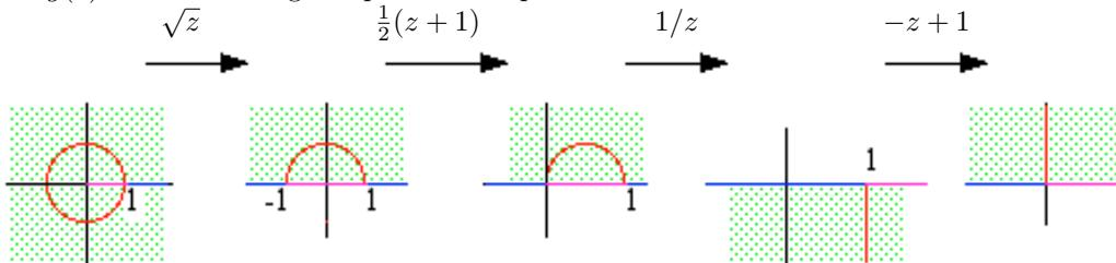
The isotherm  $u = 25$  is the image of the ray  $\theta(w) = \frac{\pi}{2}$  under the inverse map  $z = g^{-1}(w)$ ; it is the circle  $|z| = 1$ , as seen in the above diagram.
