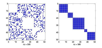
Adjacency matrix A of a graph (left), associated partitioning (right). The graph can be colored with 5 colors.
