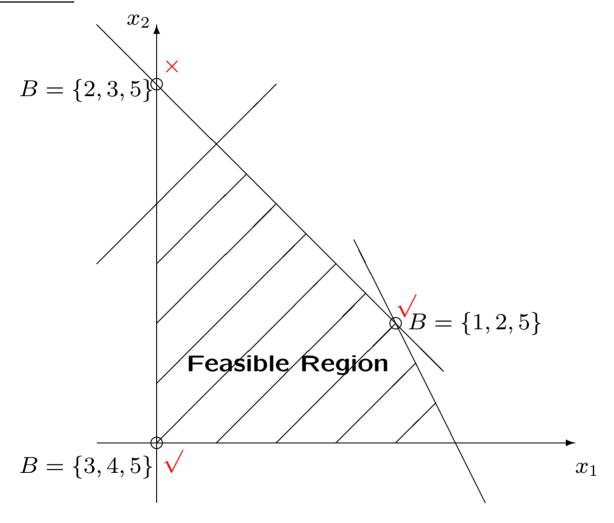
Basic solutions determined by  $B = \{3,4,5\}$  and  $B = \{1,2,5\}$  are basic feasible solutions.
