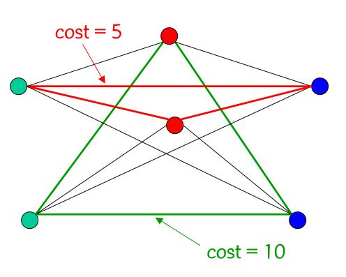
Complete tripartite graph: Each triangle made up of three distinctly colored nodes has a cost.
