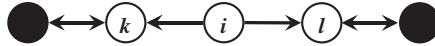
Figure 1. Example illustrating a situation occurring with PMIS coarsening, which will not correctly be treated by direct or classical interpolation. Black points denote C -points, white points denote F -points, and the arrow from i to l denotes that i strongly depends on l .
