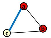
Maximum size of a matching = 1 Minimum size of a vertex cover = 2
