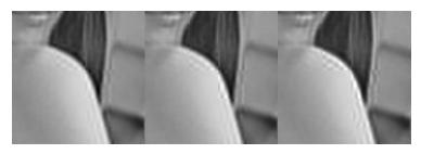
Best  $L^2$  (left), Weberized  $L^2$  (center) and Logarithmic  $L^2$  (right) approximations to Lena image using N=66 2D DCT basis functions over  $32\times 32$ -pixel blocks comprising the shoulder region of Lena image.
