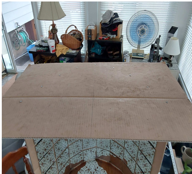
Figure 5: Photo of one of the sides of Solar Cooker No. 1 showing the positions of the nails which attach the side of the cooker to the trough. The nails are located at the endpoints of the mirrors, the linear “pieces” which interpolate the cross-sectional formula y = f(x) = x^2 .
