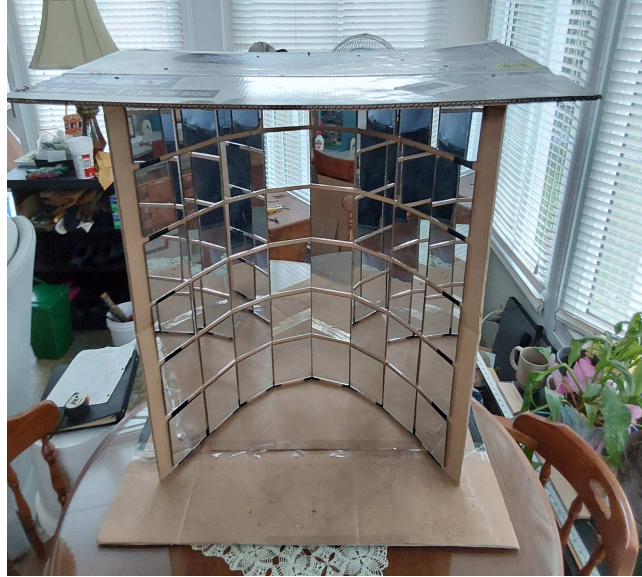
Figure 4: "Solar Cooker No. 1: Parabolic trough with cross-sectional formula y = f(x) = x^2 employing 4" \times 4" mirrors.
