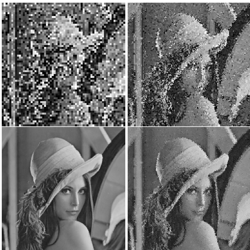
Fig. 1. Starting at upper left and moving clockwise: The iterates u_1 , u_2 and u_3 along with the fixed point \bar{u} of the fractal transform operator T designed to approximate the standard 512 \times 512 (8 bpp) Lena image. The “seed” image was u_0(x) = 255 (plain white).
