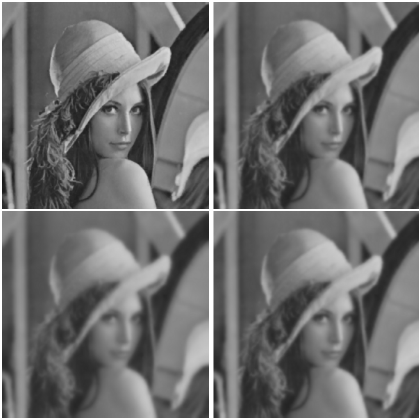
Fig. 4. Starting at upper left and moving clockwise: The limiting images u(x, t) , t \rightarrow \infty produced by integrating Eq. (2) for \epsilon values of 0.5, 5.0, 10.0 and 20.0, respectively
