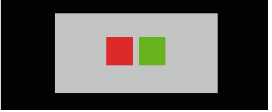
Fig. 1. Test setup for testing the impact of surround luminance on the perception of colour difference.
