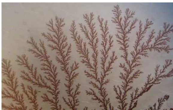
Dendritic copper crystals.
