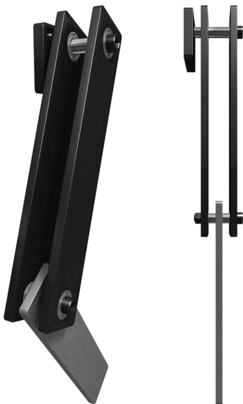
Figure 6. Three dimensional and side view of the double compound pendulum.
