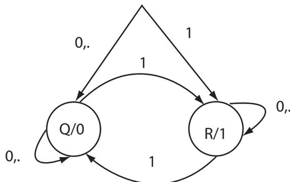
FIGURE 1. A finite state machine with input alphabet  $\{0, 1, .\}$  and output alphabet  $\{0, 1\}$ .
