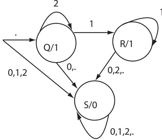
FIGURE 2. A finite state machine which produces a Saguaro set.
