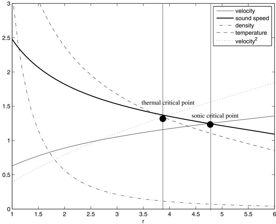
**Figure 3.** Radial transonic flow solution for  $q_{heat}(r) \equiv 0$  and  $\kappa(T) \equiv (T/5)^{0.72}$ . The two critical points are indicated. The rightmost critical point is the well-known sonic critical point, while the leftmost critical point is the thermal critical point that is introduced by including the heat conduction term. The location of the thermal critical point  $r_{crit} \approx 3.87$ , its temperature  $T \approx 1.34$ , and its velocity  $u \approx 1.16$ .
