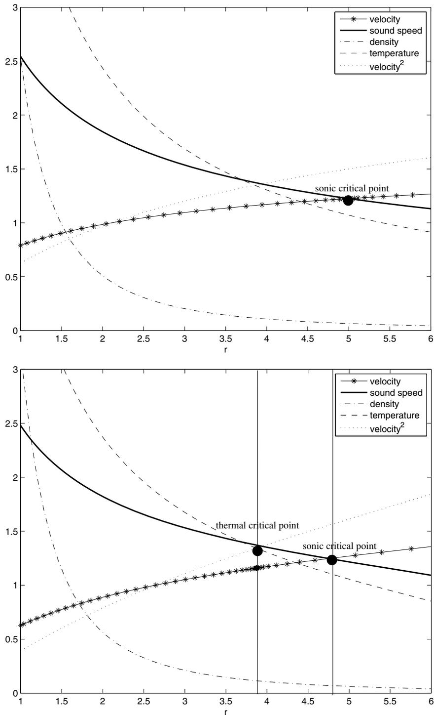
**Figure 6.** Radial outflow trajectories without and with heat conduction. Top: Radial transonic flow solution for  $q_{heat}(r) \equiv 0$  and  $\kappa(T) \equiv 0$ . The sonic critical radius  $r_{crit} = 5$ , and the flux  $F = 2$ . Bottom: Radial transonic flow solution for  $q_{heat}(r) \equiv 0$  and  $\kappa(T) \equiv (T/5)^{0.72}$ . The thermal critical point has critical radius  $r_{crit} \approx 3.87$ , temperature  $T \approx 1.34$ , and velocity  $u \approx 1.16$ .
