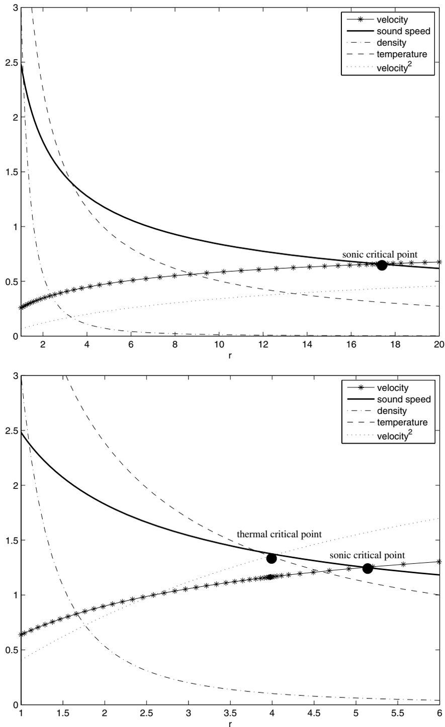
**Figure 7.** BVP flow trajectories without (top) and with (bottom) heat conduction. Both flow solutions have  $\rho = 3$  and  $T = 4.4$  at the inflow boundary. In addition,  $dT/dr = -4$  is imposed at the inflow boundary for the bottom solution. The NCP method from [14] was used to solve these BVPs numerically.
