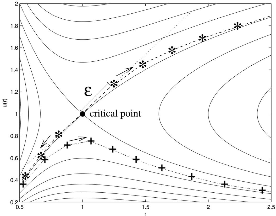
**Figure 5.** Solution curves  $u(r)$  for the spherically symmetric isothermal Euler equations with  $GM = 2$  and  $c = 1$ . Numerical integration from the left boundary (dash-dotted curve) does not allow approximation of the transonic solution, but integration in two directions outward from the critical point allows numerical approximation of the transonic solution. The arrows indicate the direction of numerical integration.
