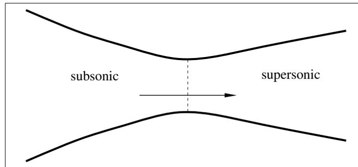
**Figure 4.** Transonic flow in a converging-diverging nozzle.
