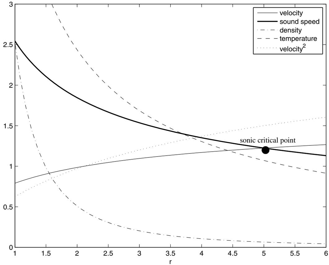
**Figure 2.** Radial transonic flow solution for  $q_{heat}(r) \equiv 0$  and  $\kappa(T) \equiv 0$ . The critical radius  $r_{crit} = 5$ , and the flux  $F = 2$ . The sonic critical point is indicated.
