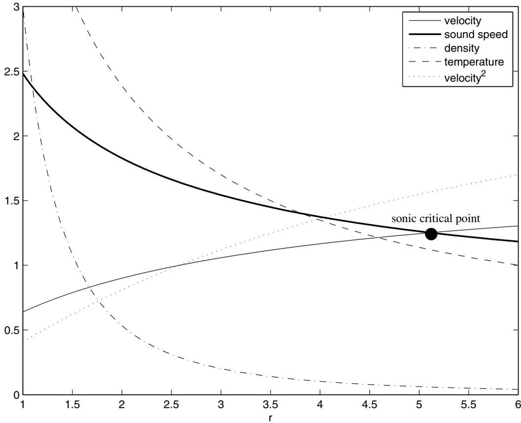
**Figure 1.** Radial transonic flow solution for  $GM = 15$ ,  $q_{heat}(r) \equiv 0$ , and  $\kappa(T) = (T/5)^{0.72}$ , and with boundary conditions  $\rho = 3$ ,  $T = 4.4$ , and  $dT/dr = -4$  at the inflow boundary  $r_a = 1$ . The sonic critical point is indicated.
