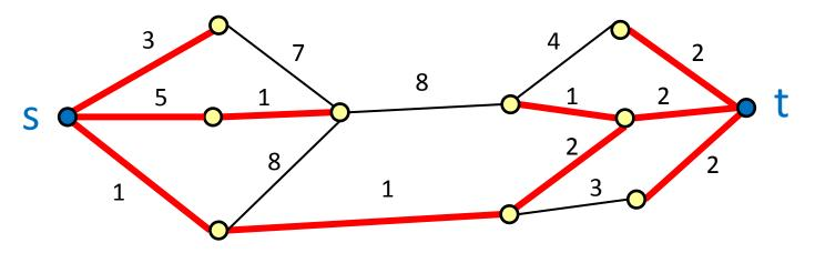
These edges are a **minimum spanning tree** There is an s-t path in the tree
