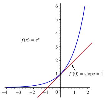
If  $f(x) = e^x$ , the slope of the tangent line at x = 0 is
