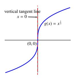
The graph of  $g(x) = x^{\frac{1}{3}}$  has a "vertical tangent line" through (0,0) which is not permitted. In fact, this "vertical tangent line" is simply the y-axis, or the line x = 0. Moreover, this line is the reflection through y = x of the x-axis which is in turn the tangent line to  $f(x) = x^3$  through (0,0).
