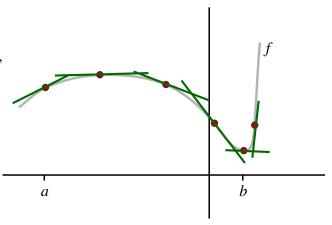
The slope of the tangent line is f'(x). Hence, the rate at which f'(x) is changing is given by f''(x). It follows that the larger the magnitude of f''(x) near x = a, the greater the curvature of the graph and the larger the potential error in using linear approximation. This means that the size of |f''(x)| is the second factor affecting the potential size of the error in using linear approximation. This information leads us to the following theorem.
