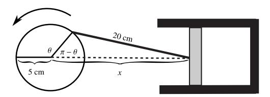
**SOLUTION** In the diagram the velocity of the piston is the rate of change of the quantity x. This means we are trying to find  $\frac{dx}{dt}$ . We also know that there are 1000 rpm with each revolution consisting of  $2\pi$  radians. Therefore, we have
