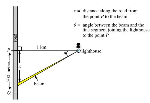
The problem asks us to determine how fast the beam is moving along the road at a particular point. In other words, how quickly is x = x(t) changing? Mathematically, we are looking for
