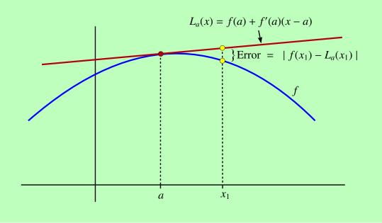
Notice that graphically, the error is represented by the vertical distance from the graph of f(x) at x = a to the tangent line  $y = L_a(x)$ .
