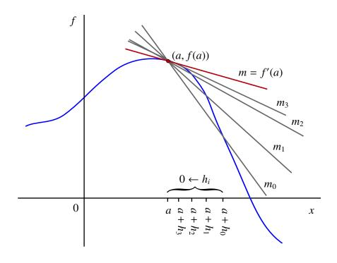
Notice that as  $h \to 0$ , the slopes of the secant lines  $m_0$ ,  $m_1$ ,  $m_2$ , and  $m_3$  are getting closer to m. In the diagram, this is represented by the secant lines visually "converging" to the line passing through (a, f(a)) with slope m = f'(a). That is, we can view the line passing through (a, f(a)) with slope m = f'(a) as a "limit" of secant lines passing through (a, f(a)). We call this line the *tangent line* to the graph of f at x = a.
