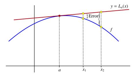
As this diagram illustrates, in principle, as the distance from x to a increases, so does the *potential* error in using  $L_a(x)$  to approximate f(x). However, it is not always true that the value of the error gets larger as the distance from x to a increases. Consider the following diagram:
