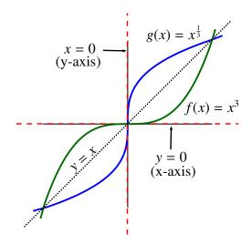
In summary, if the original function has a horizontal tangent line, that is if f'(x) = 0, then the reflection becomes a vertical line which is not permitted as the tangent line of a differentiable function. This explains why we do not allow f'(x) = 0 in the statement of the Inverse Function Theorem.
