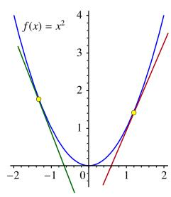
We can use first principles to find the value of the derivative of  $x^2$  at any point x:
