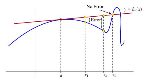
In fact, at  $x_3$  the linear approximation gives us the exact value of the function (no error). Situations such as this are uncommon. Generally speaking, the closer we are to a, the more confidence we will have in the accuracy of the estimate.
