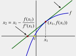
**Step 3:** We now repeat the procedure, replacing  $x_1$  by  $x_2$  and using the linear approximation at  $x_2$ , to get a new approximation
